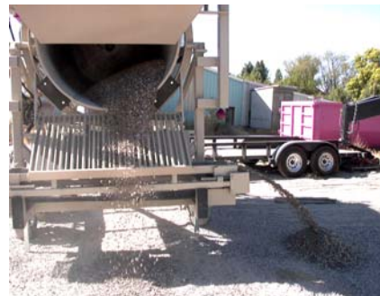
Figure 8 (waste grate & waste conveyor)
